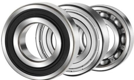
For example, open bearings are used in high-temperature applications and closed bearings in applications like sandblasting, where the bearings are protected against fine particles that could potentially clog the bearings.
